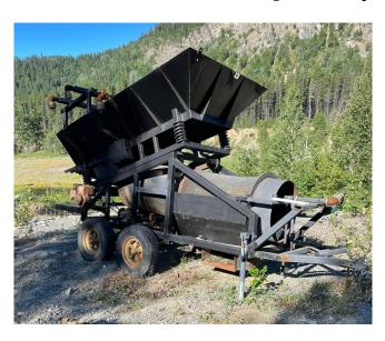
28in Dia. Gold Trommel Wash Test Plant
