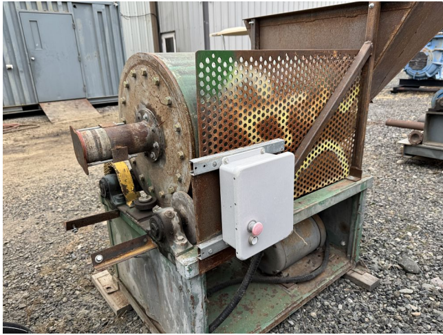
24in Dia. x 36in Long Ball Mill
