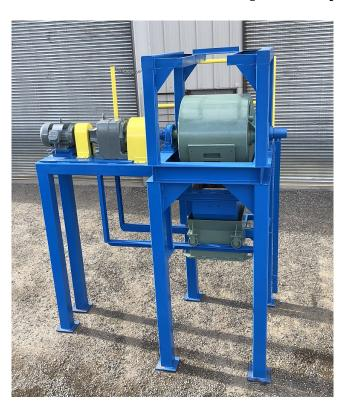
30in Dia. x 24in Batch Mill
