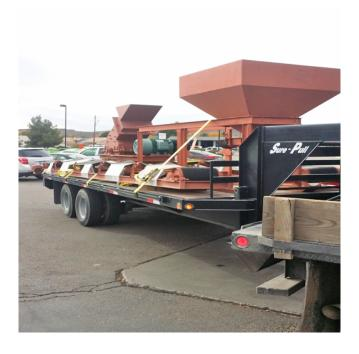
Complete crushing package consisting of Hopper, 2 TPH Fine Ore Feeder, 16 in. x 18 ft. Conveyor, and 24 in. x 16 in Hammer Mill. Includes the 25 ft. Sure-Pull Gooseneck Trailer.
