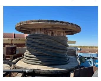
2 AWG 3C MV105 15kV EPR/PVC Power Cable
