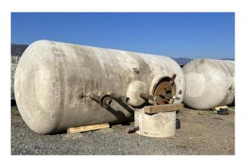
(2) 20,000L Underground Fiberglass Fuel Tanks
