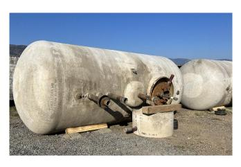
(2) 20,000L Underground Fiberglass Fuel Tanks
