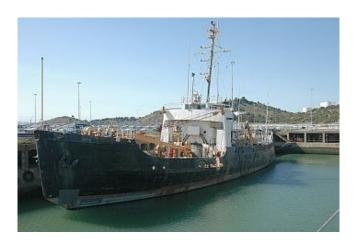
180ft EX Coast Guard Buoy Tender. Built in 1943. Overhauled by the US Government in 1988. V8-645 EMD Main engines. Accomodations for 75
