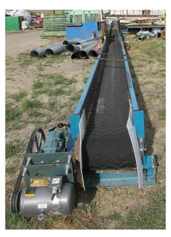
18 Inch x 58 Feet Troughed Channel Conveyor
