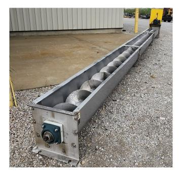
16in Dia. x 33ft Long Orthman Screw Conveyor
