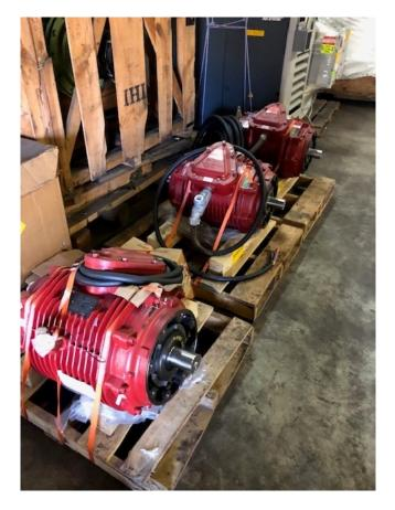
15HP General Kinematics Vibrating Feeder Motors
