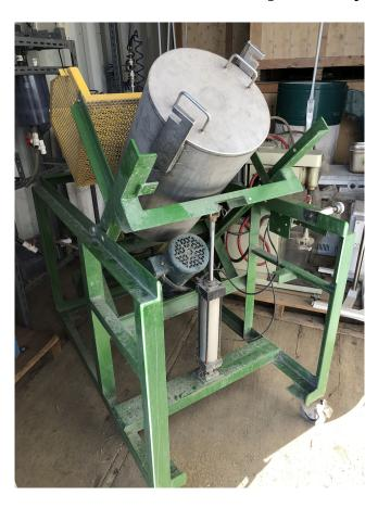
14in Dia x 21in Long Batch Rod Mill
