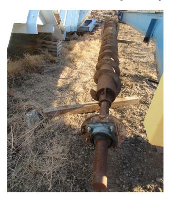
13in Dia. x 13ft Long Auger Shaft
