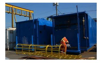
100m<sup>3</sup> Double-Wall Portable Water Tanks
