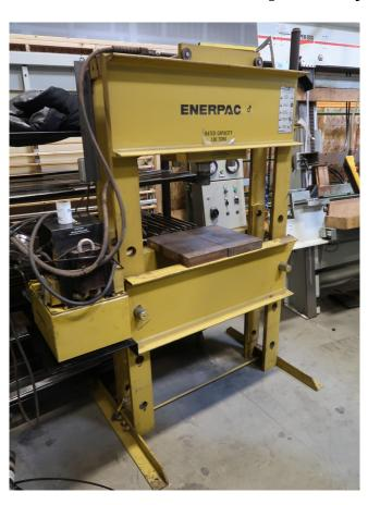
Horsepower: 1.5 HPCapacity: 100 tonVoltage: 115 VoltsSingle Phase
