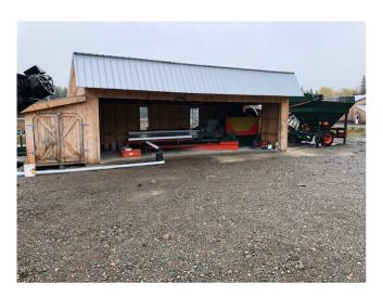
Gold Recovery Plant designed for small operation taking ore through the crushing grinding process onto the tabling of the fines to extract and recover the coarse and fine gold component in a concentrate which would be ready for refining.
