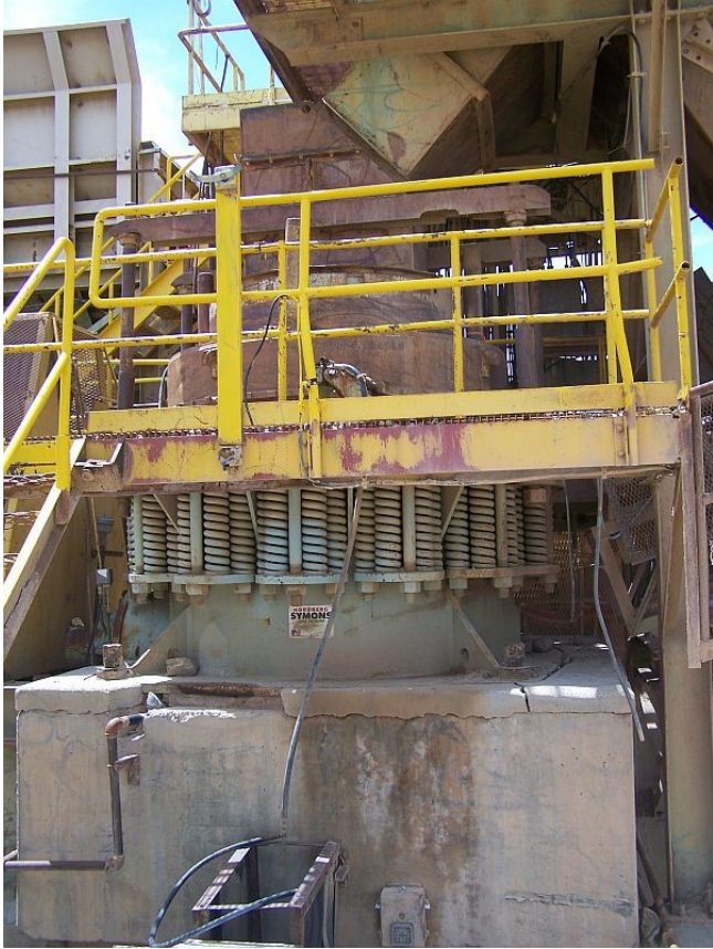
Used Symons 5.5 ft. Shorthead Cone Crusher. Hydraulic Adjust. 200 HP Motor
