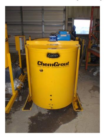
Unused Surplus Chemgrout Mixer Tank and Pump Package. 1 - Chemgrout Twin Mixer and Tank. 404 Gallon Capacity. 2 Mixers. 3 in. Dishcharge on each sides. 1 - Chemgrout Mixer Tank with Pump. 25 HP Motor Driving 4 in. x 3 in. Pump. Can be Sold Separately.
