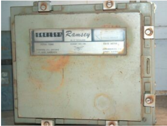
Ramsey belt scale. For 18 in. conveyor
