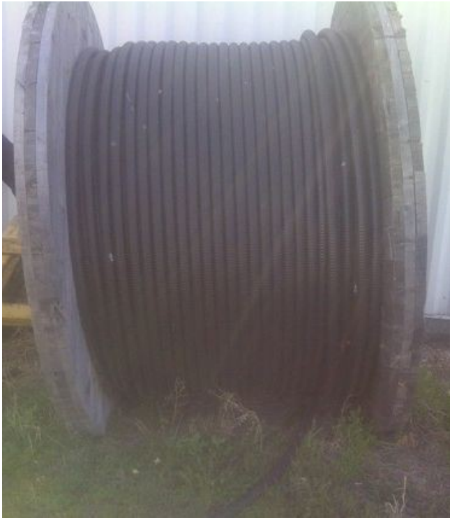
New Teck Cable. 3 OT - 3 Conductor. 2,500 ft. Spooled on Roll.
