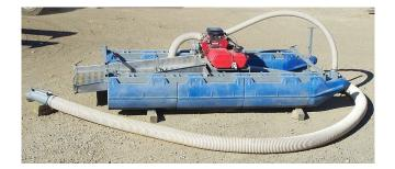
Dahlke Dredge Mfg. 7 inch floating dredge. Comes with 20hp gas drive pump and gast oil free air supply compressor.
