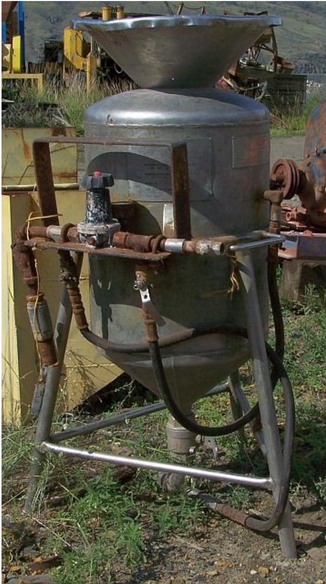
CIL Model 120 Blasthole chargers. Mounted on tri pod stand.
