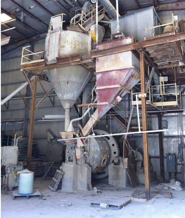
7 ft. Dia. x 4 ft. Hardinge Conical Mill. Complete with Air Sweep System.
