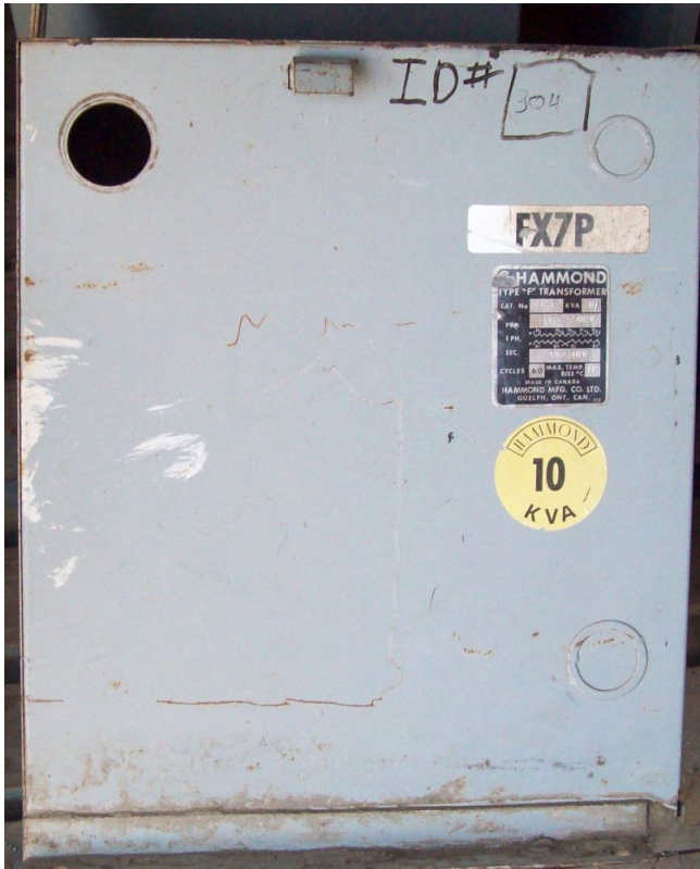
10 KVA 480 - 120/240 Single Phase Indoor Dry Hammond Transformer
