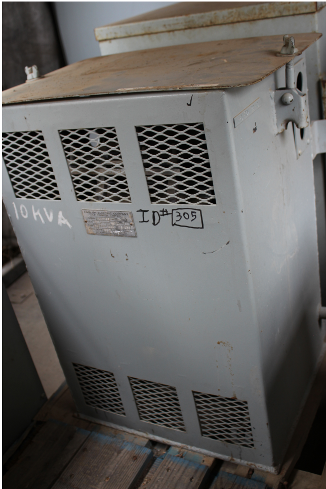
10 KVA 440 - 115/230 Single Phase Indoor Dry English Electric Transformer
