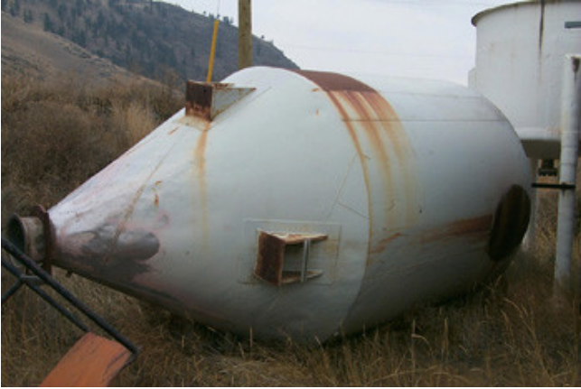
Used Stainless Steel Cyclone. 8 ft. x 14 ft.
