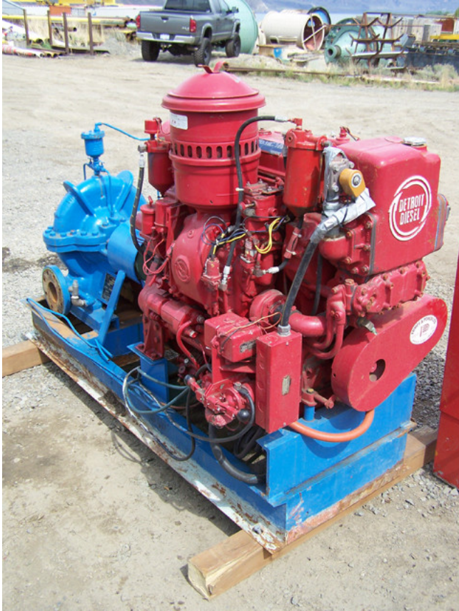
Used Detroit Diesel Fire Pump. 5 x 4 x 16 in. Impeller. 250 GPM. 100 PSI.
