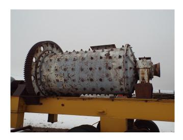
Used Ball Mill Available. 5 ft. dia. x 10 ft. Long. Steel Wave Style Liners. Belt Drive Pinion Shaft. Straight Cut Bull & Pinion Gear. 150 HP Electric Motor.
