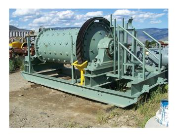
Used Allis Chalmers Ball Mill. 4 ft. dia. x 8 ft. Long. 60 hp Motor & Gear Reducer. Rubber Lined Shell. Steel Lined Heads. All Mounted on Common Skid.
