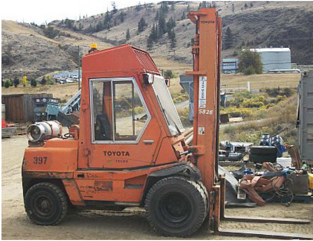
Toyota 10,000 lb. Dual Wheel Fork Lift. Propane Operated.
