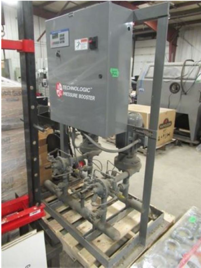
Technologic Pressure Booster Pump Skid, Bell & Gossett 70M
