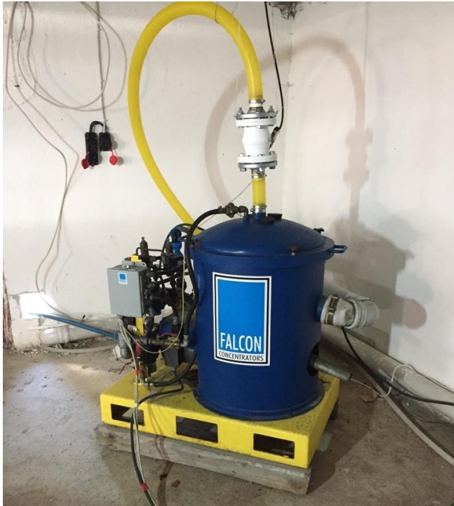
Falcon SB250 Centrifugal Gold Concentrator
