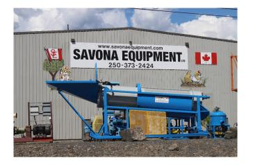
The Savona Equipment ST-Series scrubber trommel wash plants are custom designed and built as user-friendly, heavy duty, and effective wash plants. The wash plants can be operated as stand-alone processing and gold recovery systems with a sluice box or as a processing system that feeds a Hy-G Concentrator gold recovery system.
