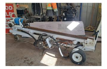
Portable Hydraulic Rock Drill
