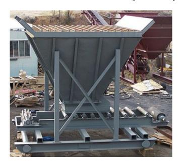
New Custom Built Grizzly Feeder. 15 Yard Hopper Capacity. 36 in. x 14 ft. Belt Feeder.
