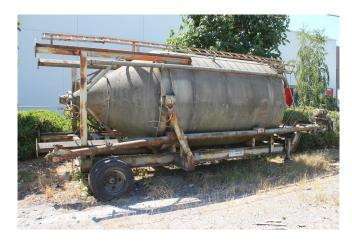
• Portable silo mounted on chassis.
