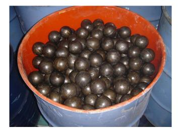
Steel Grinding Balls are stored in drums and in good condition.
