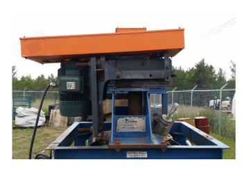
Falk 4315J05C Shaft Mounted Reducer with Motor
