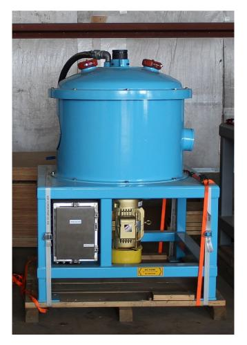
• Falcon (Sepro) UF600 Centrifugal Gravity Concentrator.
