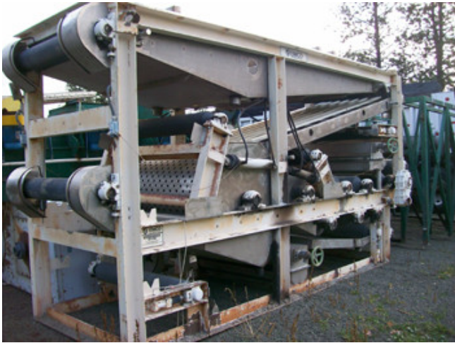
Eimco Wastewater Belt Filter Press. 44 in. wide x 15 ft. Long. Hydraulic Drive.
