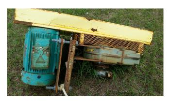
Dodge TXT715T Shaft Mount Reducer with 30HP Motor
