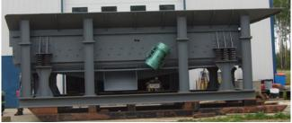
"Brand New" Gold Placer Feeder Wash Plant. 4 ft. x 22 ft. Deck. 150 to 200 Yards Per Hour.
