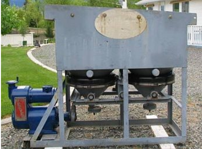
American Balanced 26 inch X 26 inch Duplex Jig.Comes with reeves vari-speed drive
