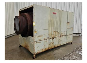
Almco 36-144MD-G Gas-Fired Rotary Drum Dryer
