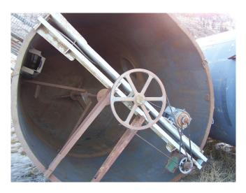
Size: 4,512 US. Gallons8ft. dia. x 12ft. Mixing Tank
