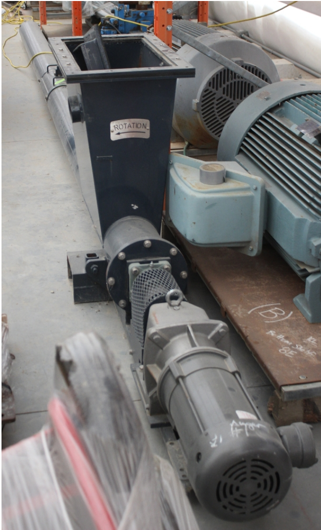
6in Dia. x 20ft Long Screw Conveyor
