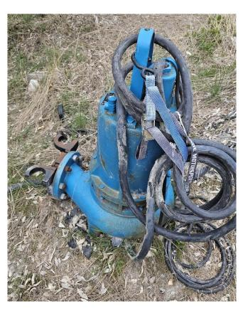
4in Barnes 4SE7524L Submersible Sewage Ejector Pump
