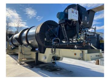
300TPH Portable Counterflow Drum-Mix Plant
