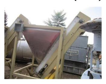
25ft<sup>3</sup> Stainless Steel Hopper with Inclined Belt Discharge
