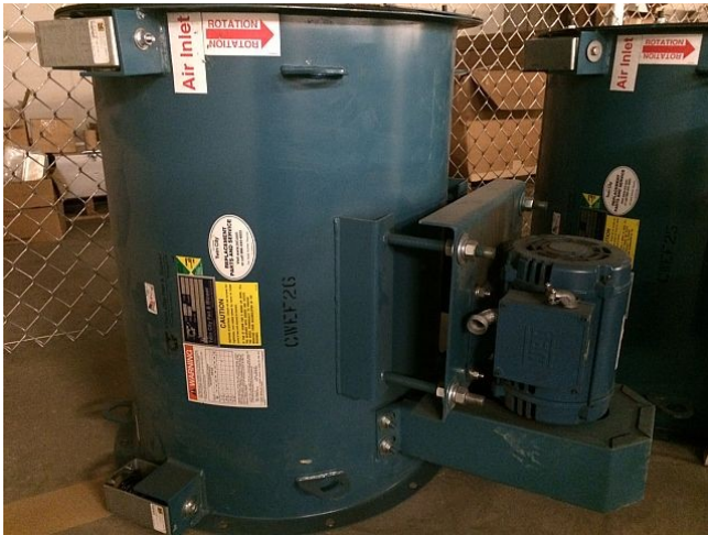
24 inch dia. Twin City Fan & Blower company ventilation fans. Model 182 TSL. Belt drive motor.
