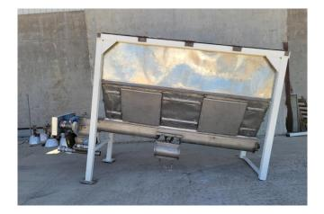
200ft<sup>3</sup> Stainless Hopper with Auger Discharge
